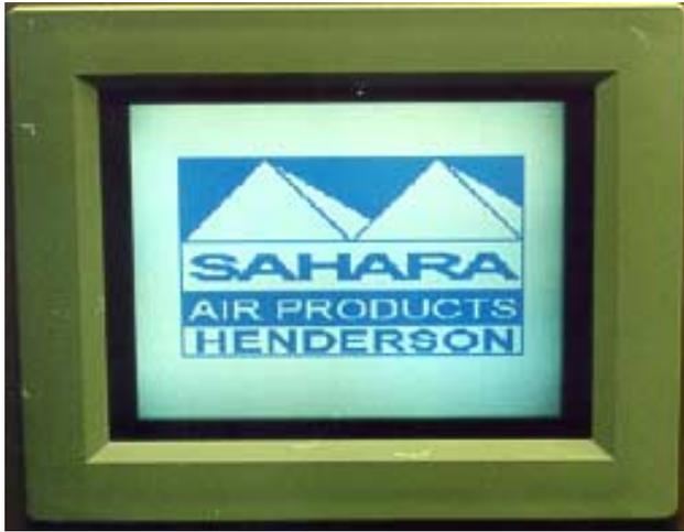
The control system for the HC dryer with the optional stripping heater and heatless mode of operation is a programmable controller with a touch screen display. The PLC controls all operations of the dryer automatically, integrating with the optional Dew Point Demand System to provide the ultimate in user friendly controls. The DPDS indicates the exact outlet dewpoint of the dryer at all times and allows the dryer to shift towers on dewpoint, rather than time.
