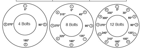
Reference the next page for continuation of the flange bolt torque procedure.
